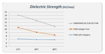
A relevant advantage offered by VAMPAMID 66 2530 V0 P GW is given by the **significant reduction of component costs compared to PA66 with halogens** due to a very competitive price and a lower density.
